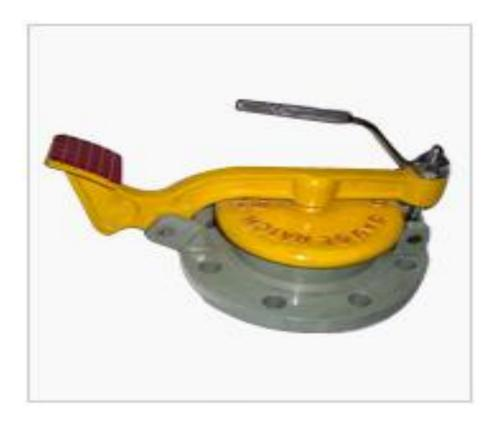
Made of quality material and components, our gauge hatch is used for controlling evaporation process and for dip measurement or for sampling purpose. Placed on the top of the tank, these hatches can easily be opened by pressing the latch with hand or foot. Our range of Gauge hatch is provided with bleeder attachment that makes it possible to relief pressure before opening the tank.
